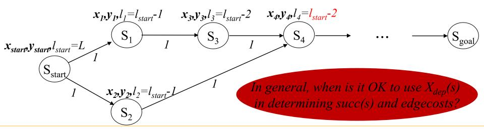
• Suppose we are planning 2D (x,y) path for UAV
