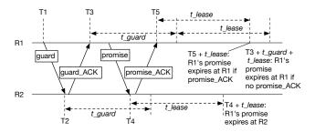
Figure 4: When clocks are not synchronized, the lease activating procedure uses acknowledgements to safely manage lease intervals. In this diagram, the lease duration is t Jease. A grantor (R1) will only send a promise if its guard is acknowledged by the holder (R2). The grantor can thus bound the promise duration even if the holder does not reply to the promise.
