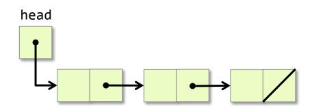
Augmenting the list with a tail pointer allows appending to operate in constant time.
