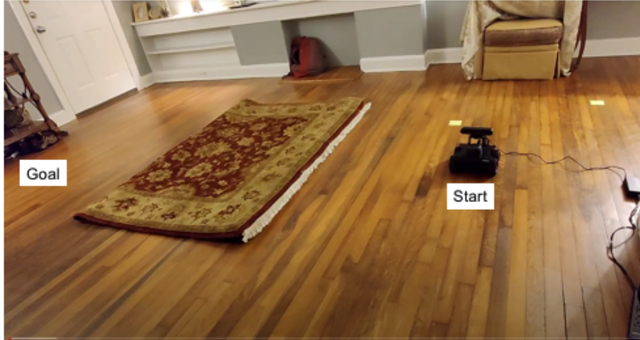
Figure 6.7: Experimental setup showing the carpet whose traversability is unknown at the time of planning, the start and the goal location.
