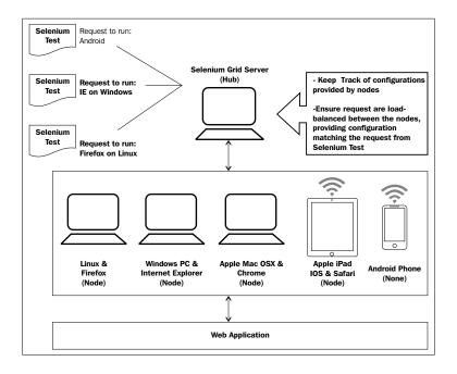
Selenium Grid allows us to run multiple instances of WebDriver or Selenium Remote Control in parallel. It makes all these nodes appear as a single instance, so tests do not have to worry about the actual infrastructure. Selenium Grid cuts down on the time required to run Selenium tests to a fraction of the time that a single instance of Selenium would take to run and it is very easy to set up and use.
