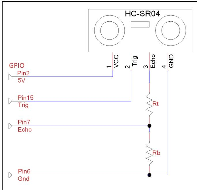
$$V_{\text{out}} = \frac{R_t}{(R_t + R_b) \times VCC}$$
