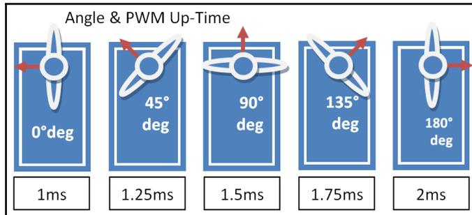
$$\text{prescale} = \left( \frac{25\text{MHz}}{12\text{-bit} \times \text{pwmFreq}} \right) + 0.5$$
