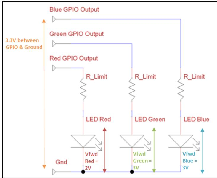
$$V_{R\_Limit} = (V_{gpio} - V_{fwd})$$
