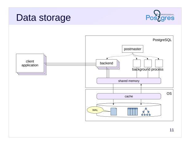
PostgreSQL works with disks on which data is located through the operating system. It almost does not use direct I/O. Data is stored in regular files and read or written using the appropriate system calls.
